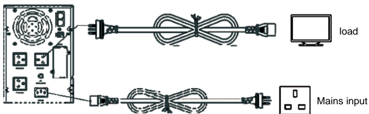
Fig. 3.2.2 Tower 500VA - 2KVA input/output connection diagram
